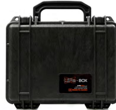
Remote Audio's MEON Series LiFe Box 20 is a Lithium Iron Phosphate (LiFePO4) battery module designed to be used as a stand-alone 12 Volt DC power source providing 250 Watt-hours (20 Amp-hours) of battery life at up to 10 Amps continuous current and digital metering all housed in a compact and portable Pelican 1150 case. The LiFe Box 20 can also be used as a supplemental battery to the MEON LiFe cart power system to extend its run time.
