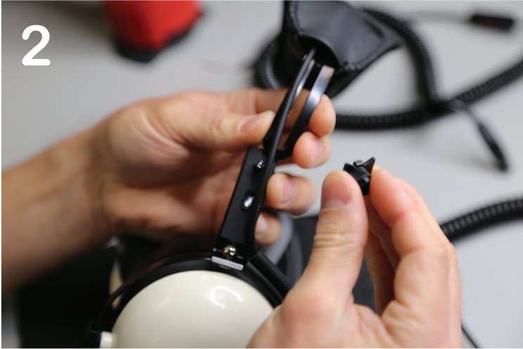
Depending on your headset, temporarily detaching the left (cable) cup from the headband will aid your work flow.
