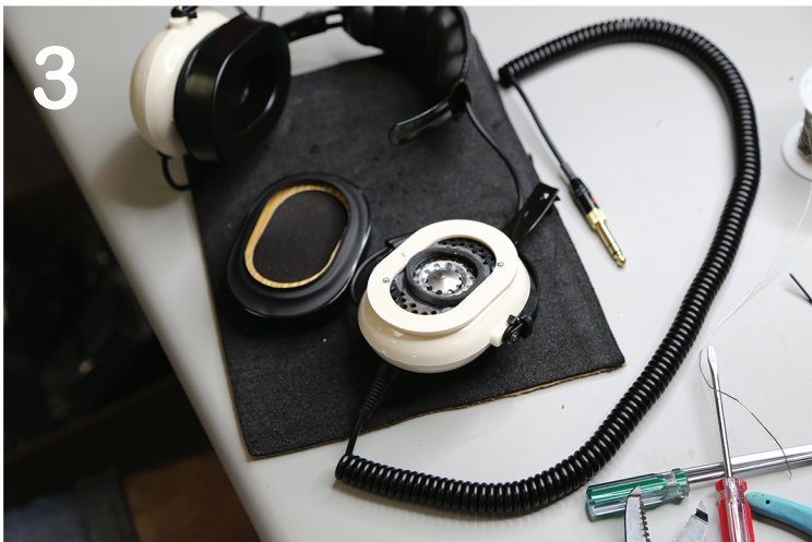
Remove the earpad from the cup to expose the driver
