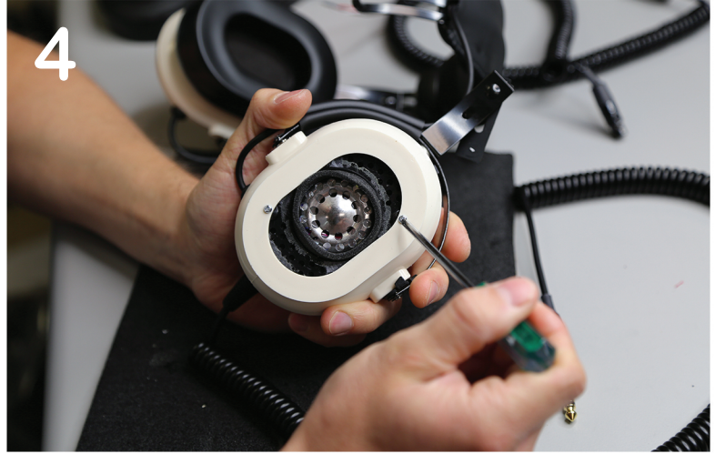
Using a screwdriver, detach the driver mount from the cup
