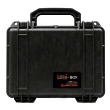
Remote Audio's MEON Series LiFe Box 30 is a Lithium Iron Phosphate (LiFePO4) battery module designed to be used as a stand-alone 12 Volt DC power source providing 375 Watt-hours (30 Amp-hours) of battery life at up to 15 Amps continuous current and digital metering all housed in a compact and portable Pelican 1150 case. The LiFe Box 30 can also be used as a supplemental battery to the MEON LiFe cart power system to extend its run time.
