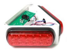
The LED lights are simple and highly programmable, with multiple patterns available. The pattern switches are easily accessed by unscrewing the rubber feet at the base of the satellites and removing the bottom plate. The main
