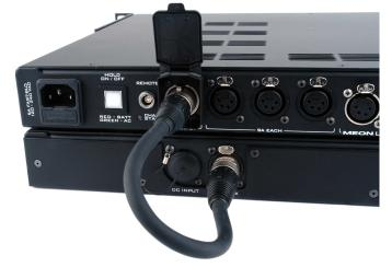
charging time will increase due to the increased battery capacity. The EL40 can be continuously charged by the MEON LiFe without risk of damage. See the MEON LiFe user guide for more information.
