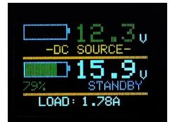
current. Using two 49Wh smart batteries in load sharing would allow up to 6.8 Amps of current draw, while two 98Wh batteries would allow current draw up to the BDSv5's overall maximum rating of 12 Amps.
