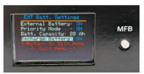
The Recharge Battery setting is used to enable recharging of a connected External Battery when the unit is on AC power. Since the internal 5Amp battery charger is designed for Lithium Iron Phosphate (LiFePO4) battery charging, it is recommended to only enable recharging on LiFePO4 chemistry external batteries. It is also important to remember that adding a supplemental battery in this fashion will increase the overall charge time of the system.
