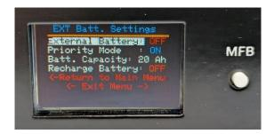
The Priority Mode setting is a new feature that allows the External battery to be prioritized for use first, thereby saving the MEON LiFe *Smart's* internal battery until the external battery voltage falls below the automatic switchover threshold.
