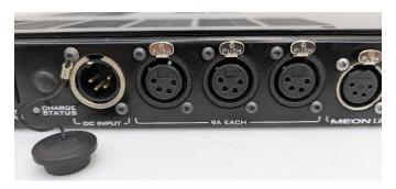
The XLR is wired in the configuration of Pins 1 & 2 (Battery -), Pins 3 & 4 (Battery +). Note, to improve reliability and reduce voltage drop, the contacts are doubled on the DC INPUT. Therefore, if the user wires their own input cables, it is recommended to connect pins 1-2 and 3-4.
