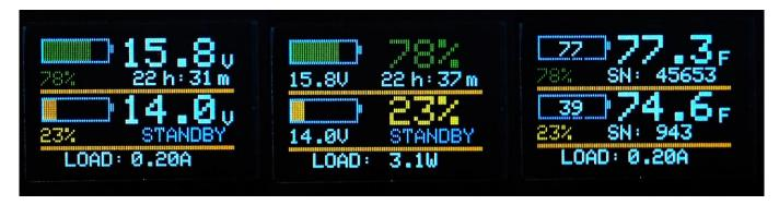
**Settings Menu:** Pressing the Menu button once while the output switch is in the "on" position (illuminated green) will enter the settings menu. Pressing the Select button will turn the highlighted setting "on" or "off". Pressing the Menu button advances to the next setting. The settings are as follows:
