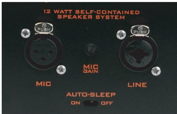
**Mic level input:** The XLR mic level input will accept a common balanced mic level signal, and will directly accommodate a dynamic microphone (powering for condenser mics is not available). One use for this input would be for a small push-to-talk cueing system. The microphone input has its own gain control, accessible on the rear panel with a small flat-bladed screwdriver.
